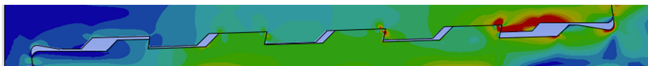
Figure 2 - A typical representation of how preload stress sits in a single start thread using heat mapping. Stresses within the connection typically concentrate near the final full wrap of the pin thread (shown on the right side of the model).
